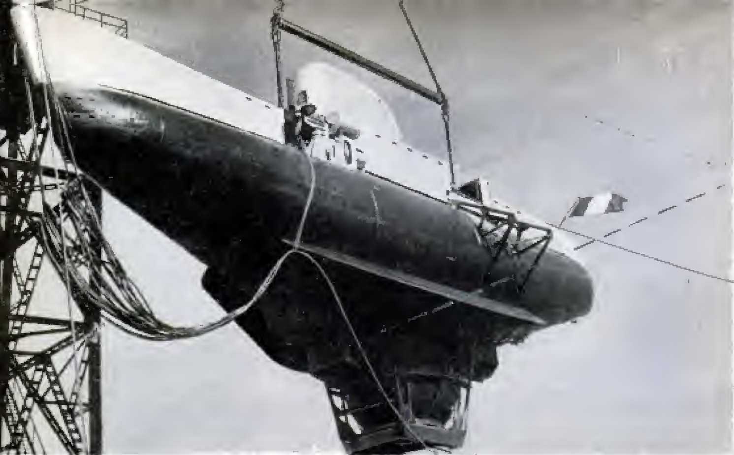
Bathyscaphe is lowered into ocean for test dive. Sphere on platform at bottom is the only watertight section
